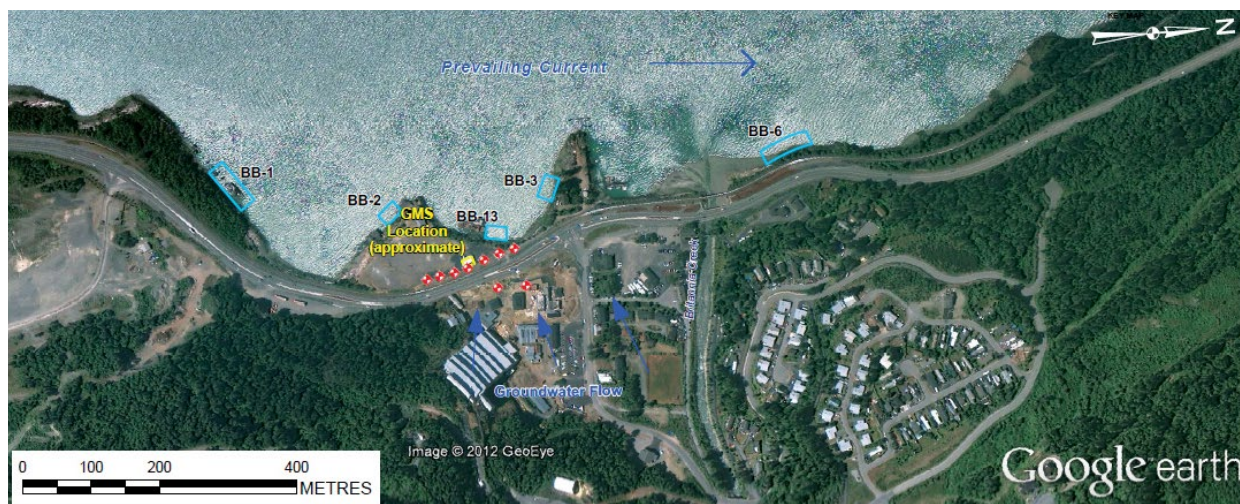
Figure 1. Satellite map of the Britannia Mine area showing sampling areas (blue boxes), including near the groundwater management system (BB-2, BB-13 and BB-3) and near-field reference areas (BB-1 and BB-6). Blue arrows show the direction of groundwater flow; red and white dots indicate extraction wells that are part of the groundwater management system. Replicated from Golder report. 4
